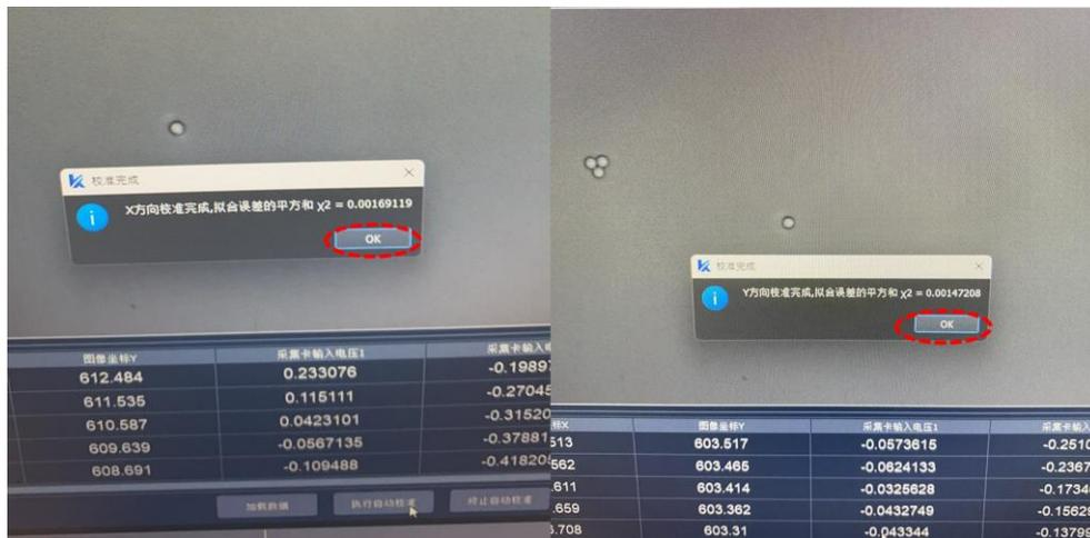
(Warning: the input voltages from capture card should linearly increase or decrease with position scanning during automatic calibration, if not, the calibration area was large than the particle.)
