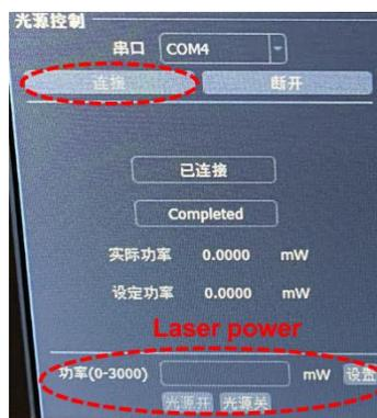
(Warning: change the 50% ND filter in the condenser to when the light power over 1000 mW to protect the QPD sensor.)
