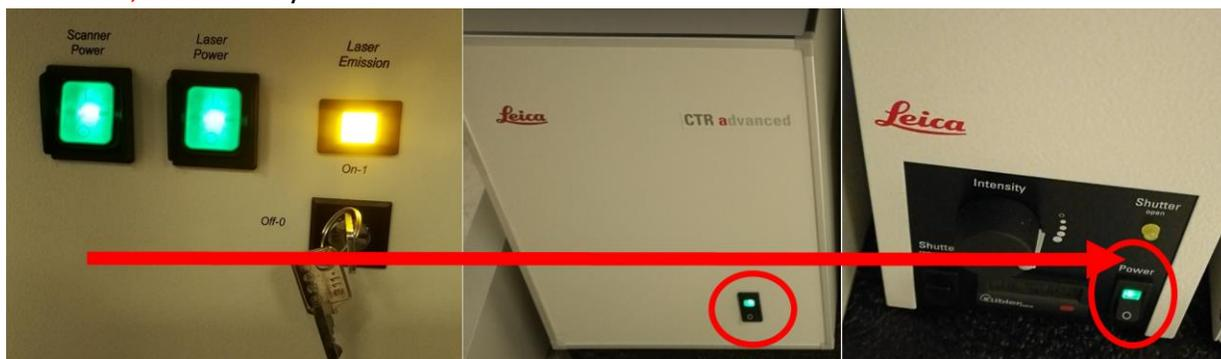
2.2 Turn on the **Fluorescence exciting light source** if necessary. (only for fluorescence imaging, **NOT** needed for confocal imaging)
