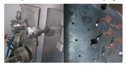
2.3 Switch the shutter to right under the sample to prevent the possible impurity evaporation at the beginning of heating.
