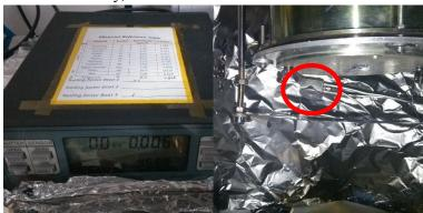
2.5 Before loading the crucibles of sample, use multimeter to measure the resistance between **the electrode connected with the boat** and **the ground**, one should be OL, the other one should be around  $0.2 \sim 20 k\Omega$ . Check all the electrodes of the three boats and make sure none of the electrodes is directly connected to the ground. If not, please contact the maintainer.
