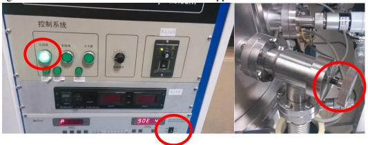
3.3 When the pressure of the chamber goes down to 15 Pa, turn off the low vacuum valve and turn on the backing valve.
