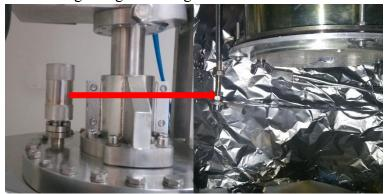
2.4 Check the crystal monitor to make sure its life is sufficient and not out of order, otherwise clean the monitor cap or replace the quartz monitor. Input the materials parameters such as density, z-vale.
