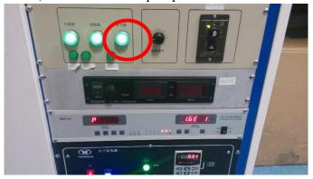
3.5 After around 1 min, open the high vacuum valve.
