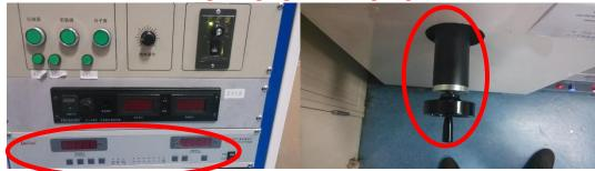
2.2 Vent the chamber by opening the valve at the corner of the chamber, clamp the samples on the sample holder and screw the holder on the top stage.
