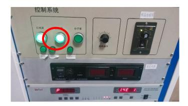
3.4 After around 1 min, turn on the turbo pump.
