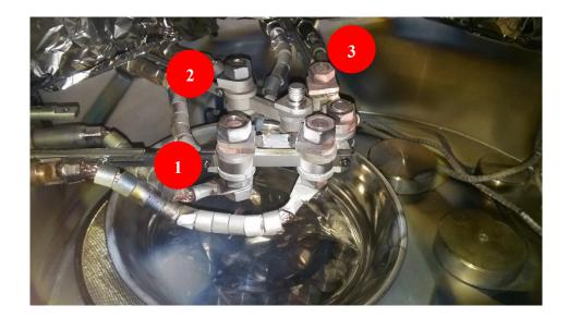
2.7 Close the door and make sure the metal plate is at the correct position, otherwise it will break the vacuum of the door; tighten the screw, make sure door is sealed.
