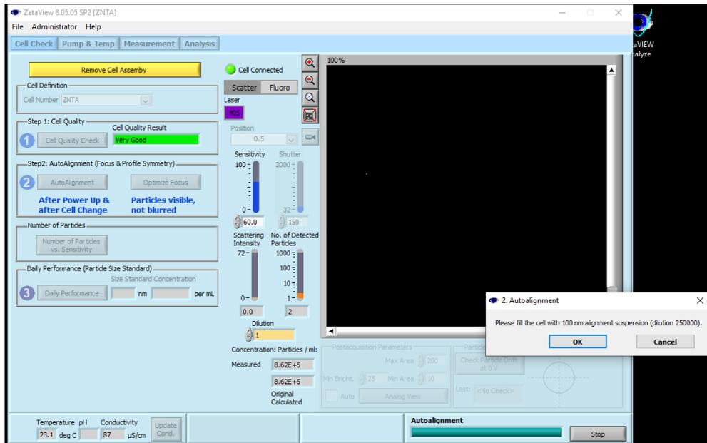
2.7 Please inject 1 ml alignment suspension and press OK. Please avoid generating air bubbles during injection.
