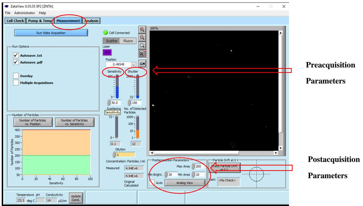
In general, the sensitivity should be adjusted accordingly depending on the scattering behavior of the sample. The shutter value means adjusting the duration of the exposure time of the camera. The indicated value is reciprocal in seconds (e.g. 1/70 sec). High values mean short exposure time, low values represent long exposure times
