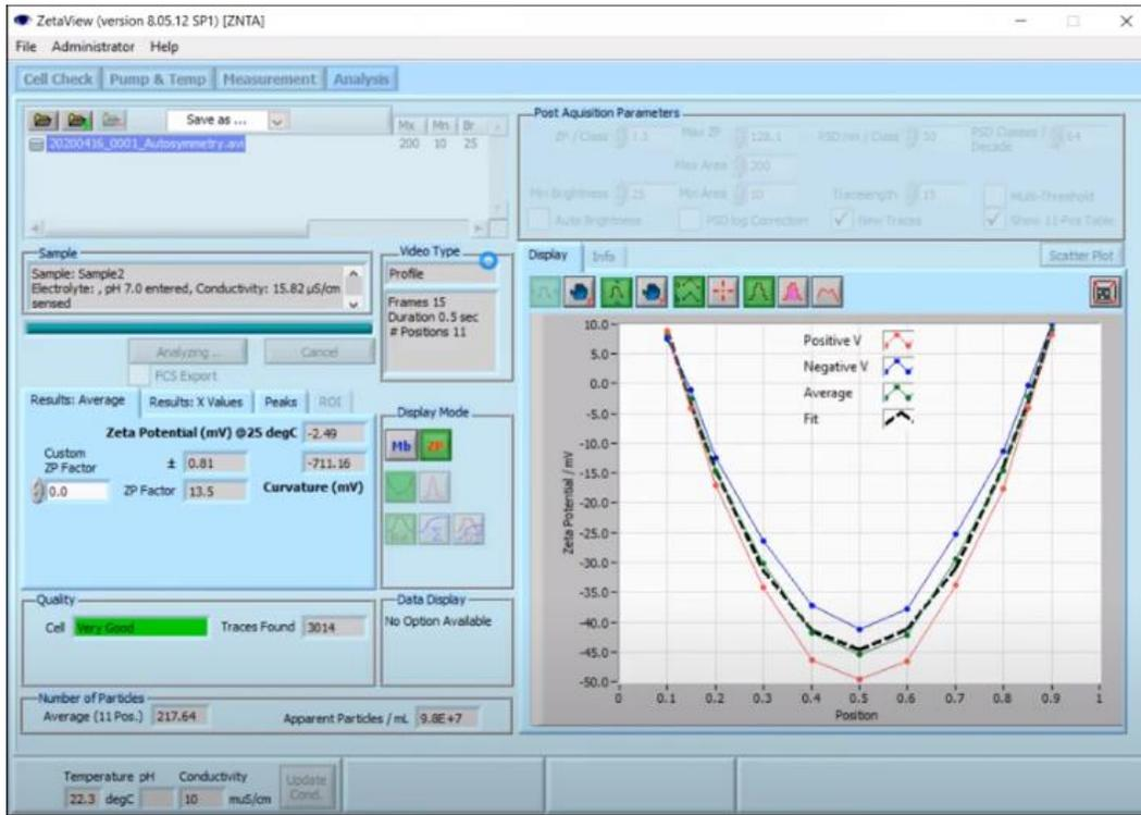
Finally, a profile symmetrization is performed which results in establishment of a parabola. The parabola shows up automatically in the “Analysis” menu and indicates the cleanliness of the measurement cell in terms of absence of dirt, air bubbles and other positive charged particles that may attach on the cell walls.
