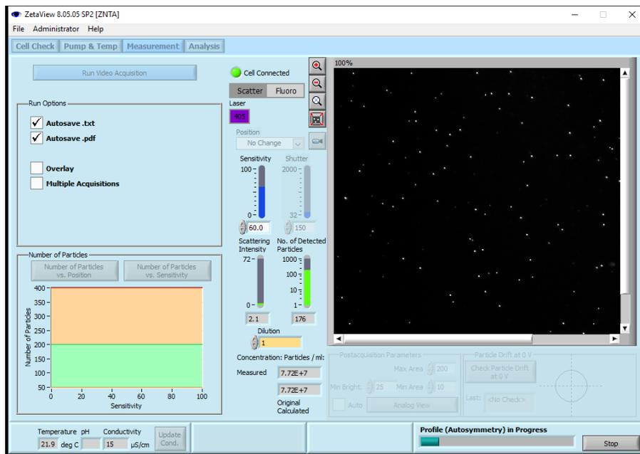
During autoalignment the instrument finds particles, focuses on the particles first in large steps followed by small steps and finally performs a zeta potential measurement for profile symmetrization (see below). The profile should be symmetric and smooth. If the curve is inverted, jagged or flat, there is air bubbles inside the cell, the cell must be cleaned.
