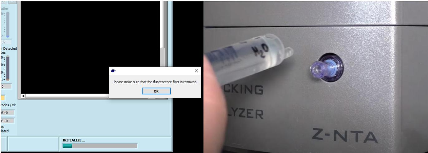
2.5 After initialization the message “Please check the fill level of the water reservoir” appears. Select **pump 1**, click **Rinse**. The ZetaView instrument performs a CellCheck (“Cell Quality Check in Progress”) which is visualized by the progress bar at the lower right of the window. During the pump rinsing process, inject 10-20ml water from the injection port to remove dead volume in the cell.
