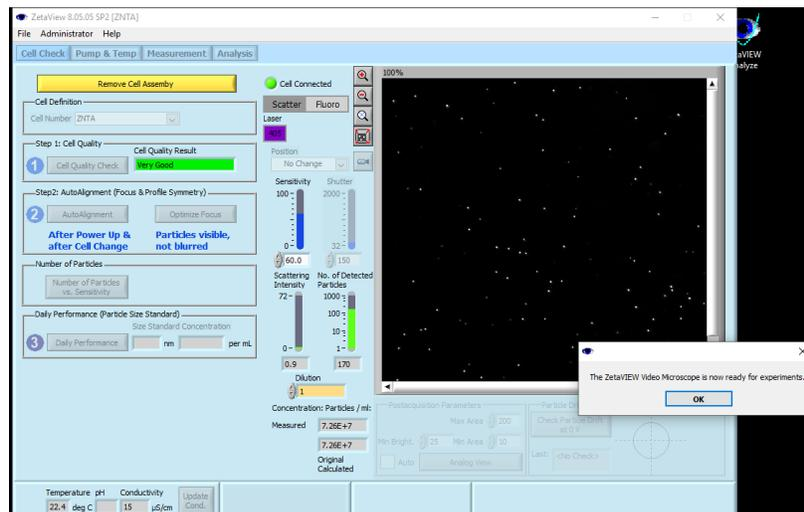
**Reminder 2:** The calibration process may fail and “Zetaview is not ready for experiments” will appear. Please **disassemble the cell and clean the cell** strictly according to the **cleaning SOP** attached. **Common users should make sure the calibration process is OK before and after your experiment to avoid any contamination of the cell. Mark down your calibration process before & after the experiments in the Notebook.** (See **Cleaning SOP** for the detailed process)
