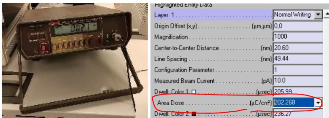
In case the beam current is shown on SEM computer but not on the external picoammeter. Click the “**Sample to external picoammeter**” in the “SEM” menu. It is recommended to use data from external picoammeter instead of internal picoammeter due to higher accuracy and reliability.
